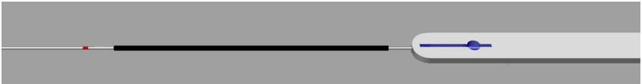
7. Now that you shortened the steel wires and glued a cf tube on 2 of the slugs insert all of them again in the model and check whether the mark still gives you the desired CG, if not put a new mark on it at the middle hole.
