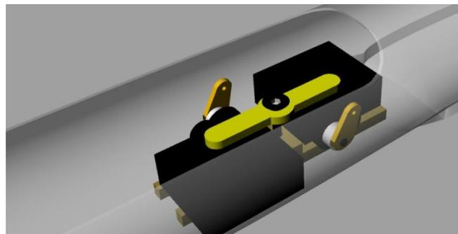
7. Cut the pushrods to length , one needs to be 145mm the other 165mm.
