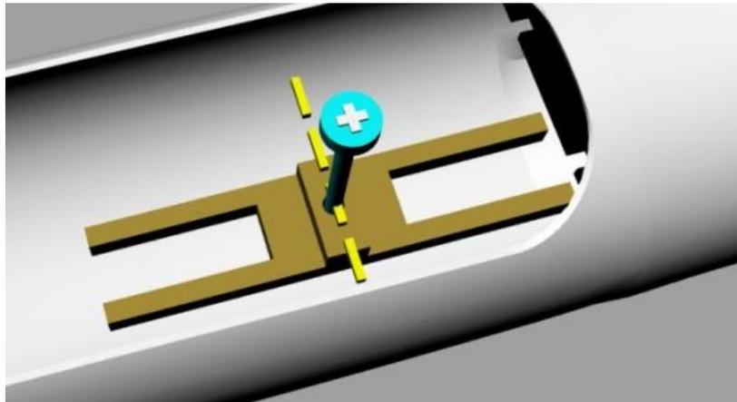
5. Glue the guidance plate into the fuselage, first sand the inside of the fuselage add a good amount of (thickend) epoxy right underneath the slot , then push down the guidance plate and let it cure.
