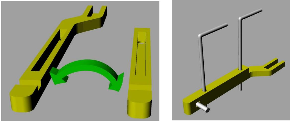
2. glue in the 3mm cf tube with thin CA , once cured wrap a thread around it (I use sewing thread) and add another drip of CA to fixate. Do this for both pushrods.(you can glue one on each end of the carbon tube)
