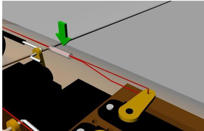
12. Center the servo in your TX, put on the servo horns 90° and pull the steering line so there is no rudder or elevator deflection, mark the steering line where it meets the servo horn hole and bend 90°, proceed like described in the tail manual and do the same for the other servo. **Use a hole 5mm out of servo center**. Slide over the plastic tube, press it with pliers and transfer a drip of thin CA to it.
