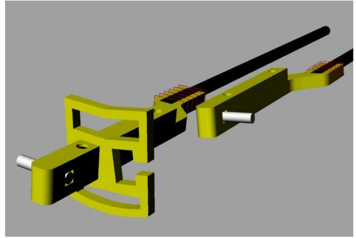
4. Put a mark (line) inside the fuselage at 138mm from the nose tip , screw the M3x25mm bolt in the servo tray (screw it in all the way , the bolt will protect the threaded hole from glue) , glue it in with epoxy , the bolt hole on the 138mm mark , make sure it runs centered and the bolt stands up straight.
