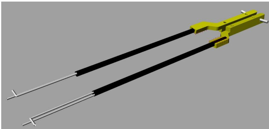
9. Attach the pushrods to the servos, bolt the wing on, make sure the fork shaped horns on the wing are placed onto the dowel pins on the pushrod and tape the ailerons at the root for 0 deflection.
